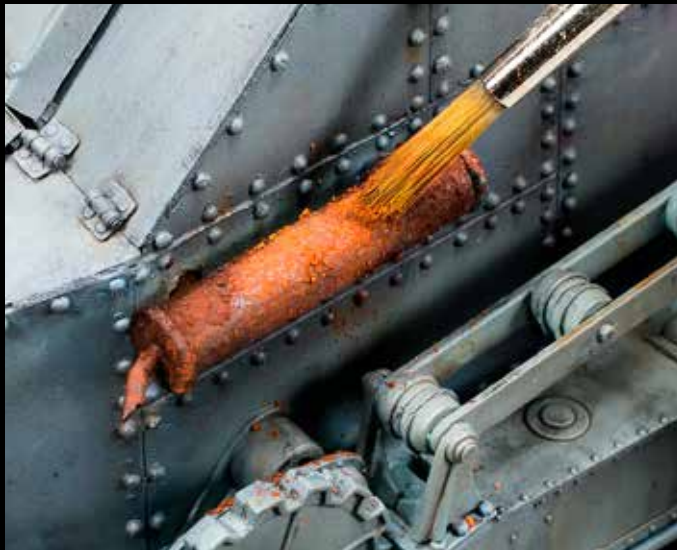
The center of the exhaust was worked with light rust pigment.
