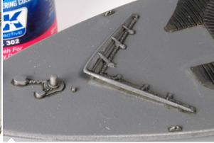
Remove the excess with White Spirit so that the darker zones match with the edges of the ship structure and assembly of the rest of the details.
