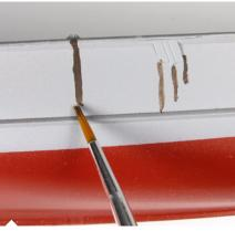
Apply the product starting from the deck or any area prone to accumulate dirt, like the drains.
