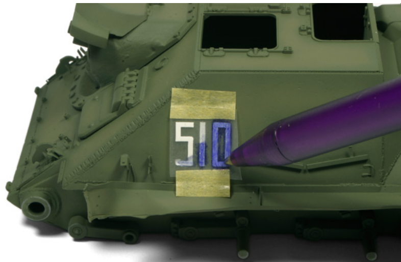
Use a pencil or a biro to rub over the dry decal until it attaches itself on your model.
