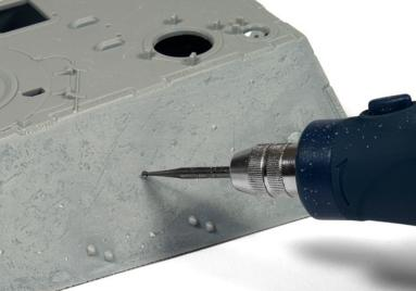
Install a small round headed bur in a motor tool and tap at low speed against the plastic, in a very irregular pattern. This way you will create a very irregular and uneven surface on the plastic.
