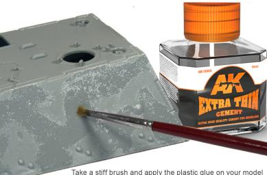
Take a stiff brush and apply the plastic glue on your model in a dabbing manner. After a few seconds the glue start to melt the upper layer of the plastic and by dabbing it in an irregular pattern the texture will appear.
