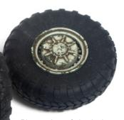
Place a drop of glue in the hole in the rim and mount the tire on the rim making sure the needle inserts the hole in the rim and add some light pressure and hold it until the glue has dried.
